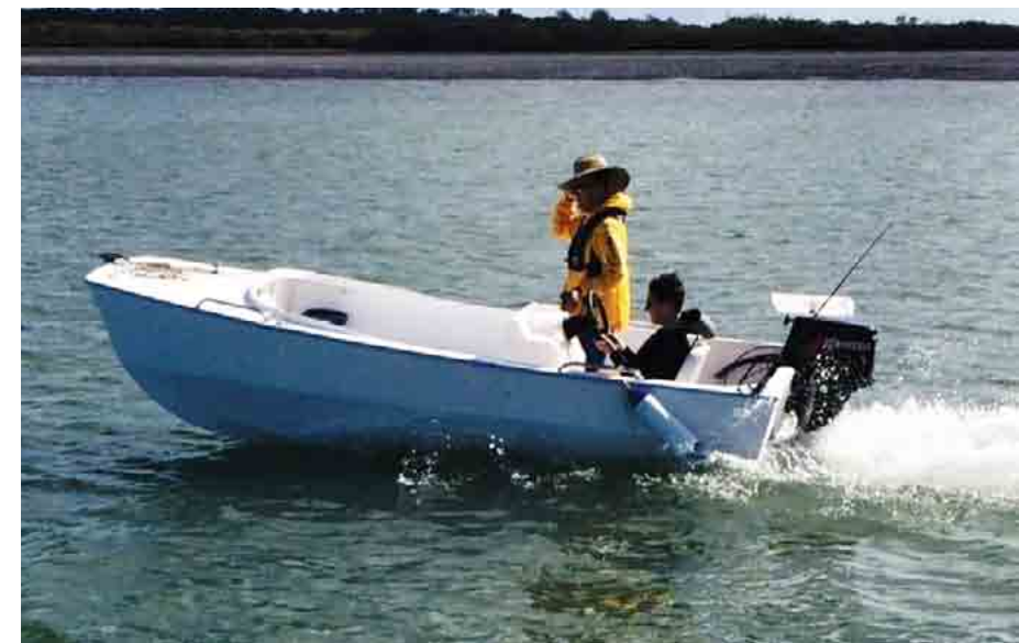
The 4.2m Ripple tender underway, this vessel fitted with a 20hp outboard.
