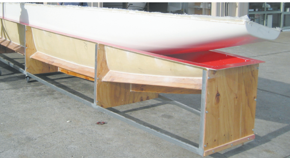
A Spirited 380 hull being produced from the female mould.
