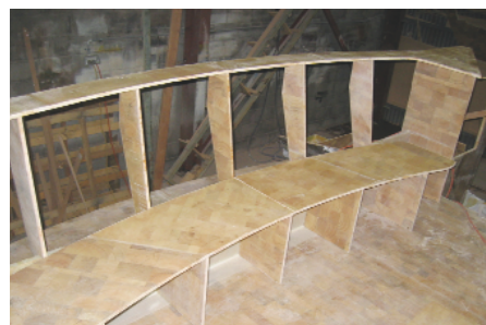
Aft cockpit seat being assembled.
