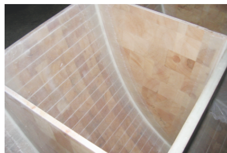
The Kerfs on the inside of the bridgedeck panel.
