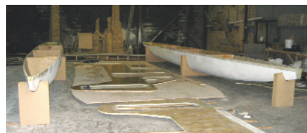
Both hulls ready for bulkheads to be fitted. Day one of assembly.
