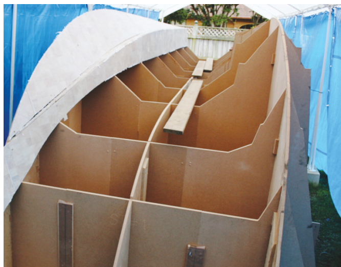
Hull panels being fastened into position.
